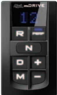
The mDRIVE is designed to integrate seamlessly with the Mack MP7 and MP8 engines in the Econodyne® and MaxiCruise® families. There's no clutch pedal, and the gearshift is operated by intelligent electronics. Any Pinnacle packaged with an mDRIVE automated manual transmission not only delivers smooth shifts every time, but it opens you up to a larger pool of drivers.
