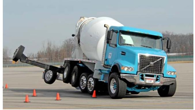
Volvo Enhanced Stability Technology (featuring Bendix® ABS-6 Advanced with ESP) provides core antilock braking, Bendix® Smart ATC, and an enhanced stability system (covering under-steer, over-steer, and rollover situations), making this the most effective ABS-based traction control and enhanced stability system on the market today.
