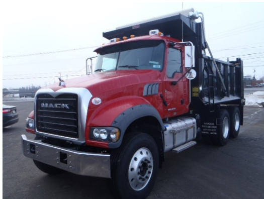
14' Heated Bibeau Model BFL-S dump body with tarp.
